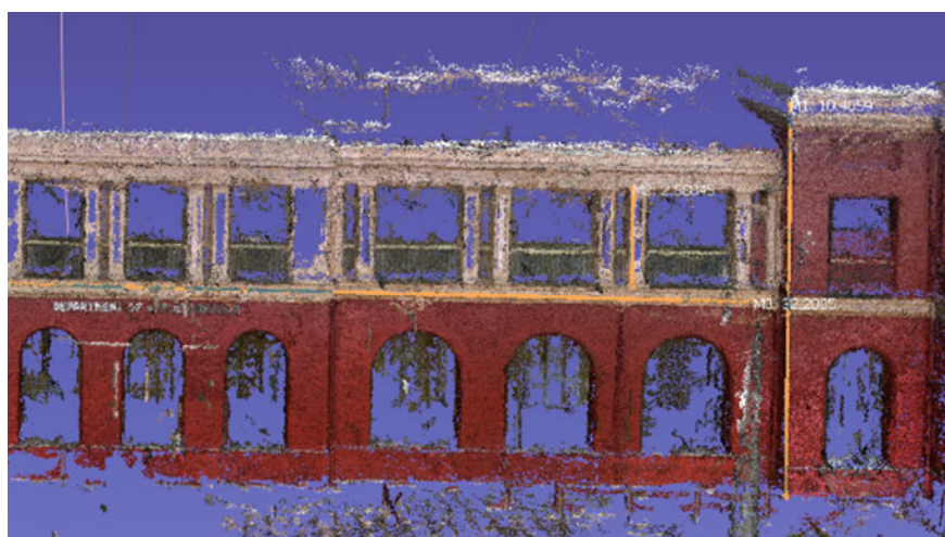
Fig. 6 Measurement is done on the 3D model created from Nokia Lumia 1020
