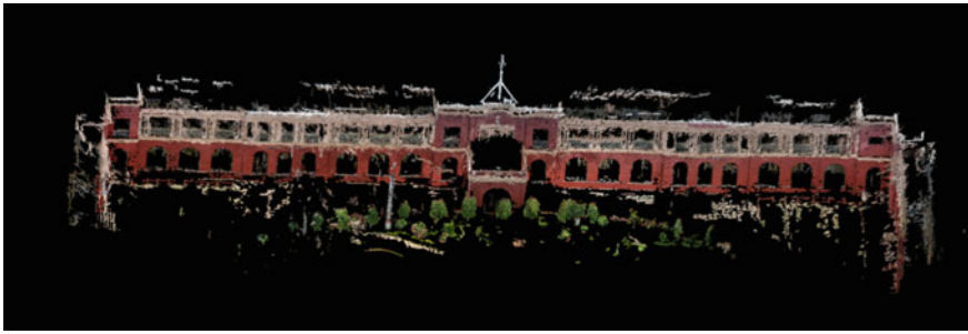
Fig. 4 Dense reconstruction made from the imagery of by Oneplus 3T
